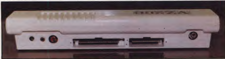
Four I/O connectors and two plug-in slots are on the back.
